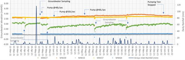
Graph 3: Groundwater level trends in the DBG / PWT aquifer (approximately 5m to 50m depth) shows response only to natural climate variations and no impact of pumping.
