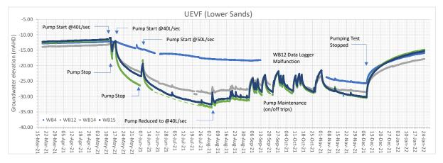
*Graph 1: Groundwater level (pressure) trends for the lower part of the UEVF aquifer (approximately 180 to 250m depth) show declines and recovery as modelled.*
