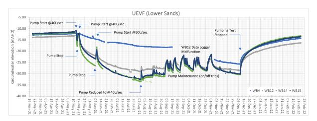
Graph 1: Groundwater level (pressure) trends for the lower part of the UEVF aquifer (approximately 200m depth) show declines as modelled.
