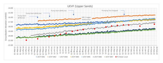
Graph 2: Groundwater level (pressure) trends for the upper part of the UEVF aquifer (approximately 40m to 140m depth) show no impact of pumping.
