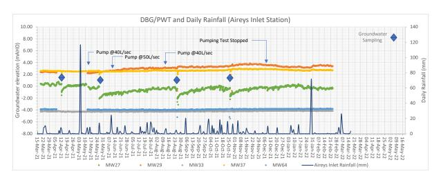
Graph 3: Groundwater level trends in the DBG / PWT aquifer (approximately 5m to 50m depth) shows response only to natural climate variations and no impact of pumping.
