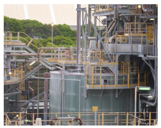
Figure 13: Liquor Burning Slurry Mixing Tank (48A)
